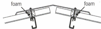
Flat Ridge Cap 150° Cross Section: Sealing with shaped foam polyethylene strips Figure 18b
