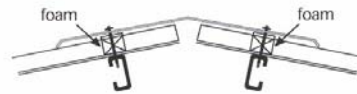
Flat Ridge Cap 150° Cross section: Sealing with shaped foam polyethylene strips Figure 18b
